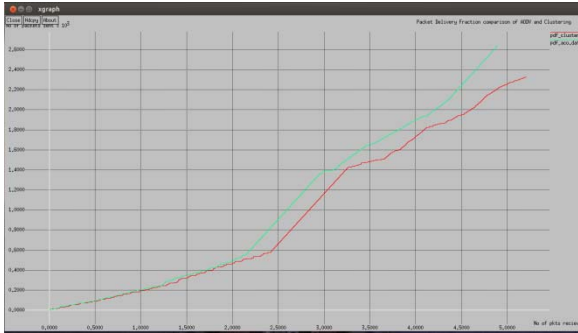
Figure 5: Comparison of PDF for cluster head communications with AODV and ACO
